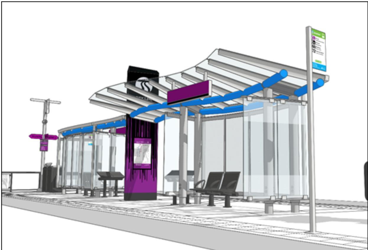
*City Line station rendering: 1rolled-tube steel highlighted in blue*
